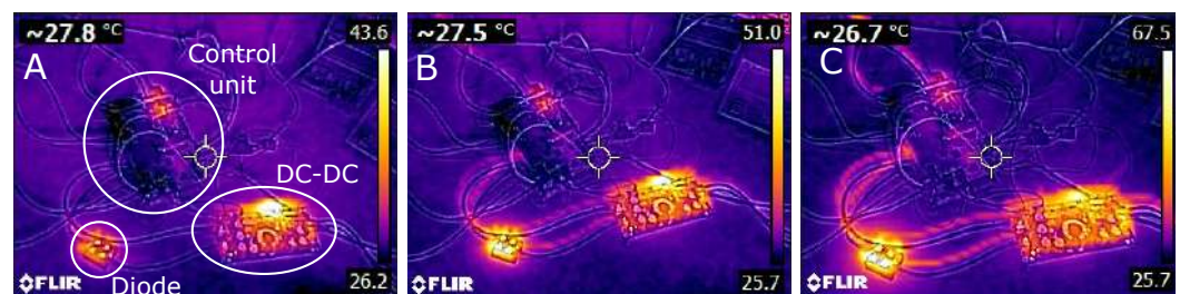
Figure 9. Images collected during the thermal test with the thermal camera: (A–C) correspond respectively to 100, 200 and 300 W of power flow.
