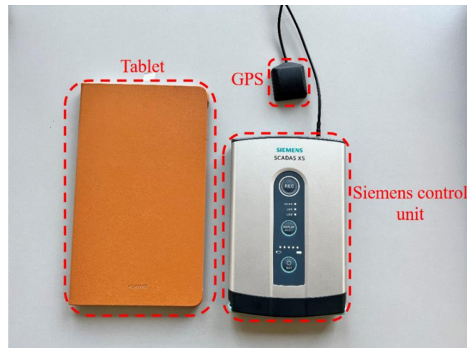
Figure 4. Instrumentation used for data acquisition. It consisted of a control unit provided by the Siemens company (model SCADAS XS Compact), a GPS sensor and a tablet for the monitoring.
