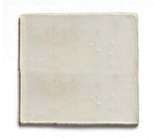
Figure 2: Samples of Transparent Wood of 5-Centimeters Squared Used During the Data Collection
