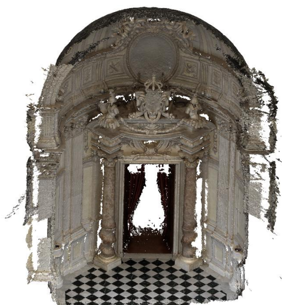
Figure 3. Dense point cloud generated using Agisoft Metashape on the portion of the Galleria Grande.
