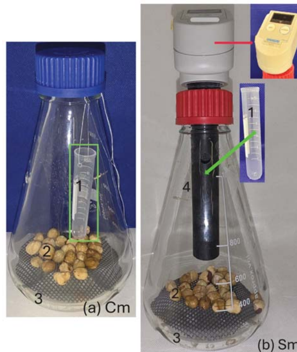
Figure 11. Cone bottles: Cm (a) and Sm (b) microcosms. (1) Tube for NaOH solution; (2) hazelnut monolayer on the plastic grid; (3) water; (4) holding tube. In (b) the respirometric sensor details are shown with a red arrow.
