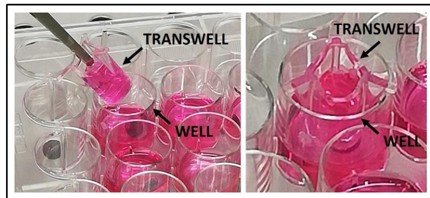
Figure 3. The set-up of the indirect co-culture with well and transwell device. The transwell has to fit perfectly into the well allowing the plate lid to close. Tweezers are used to remove the transwell from the well.
