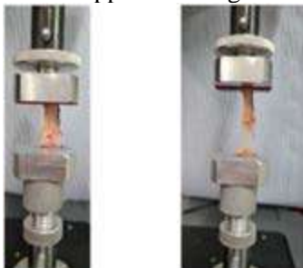
Figure 1: A. Sample set in the jaws - B. Sample after breakage.
