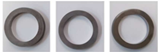
Fig. 9. Toroidal specimens after milling
