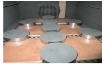
Fig. 7. Specimens of heat treatment in the oven
