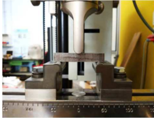
Fig. 19. Transversal break test device (TRS)
