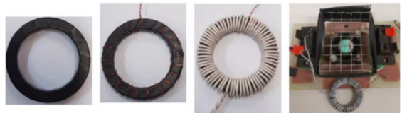
Fig. 10. Toroidal specimens with the windings required for testing
