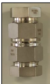
Figure 12: 10 mL bomb-type batch reactor.
