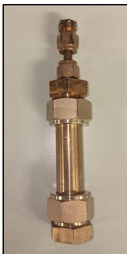
Figure 9: 20 mL bomb-type batch reactor.
