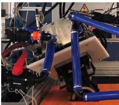
Figure 1: Stack at inclination towards the back and left.
