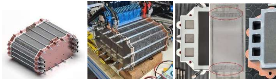
Fig.1: Virtual assembly of the stack (left), manufactured stack on the test bench (centre), gasket design modification (right)
