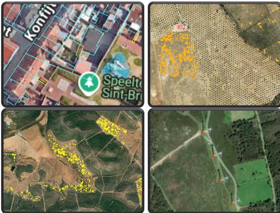
Figure 7 Examples of polygons of small size features (olive trees, wind farms) identified as false positive buildings.
