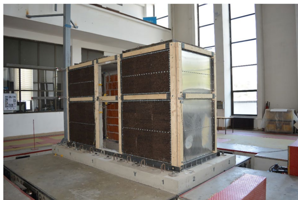
Fig. 4 RC model strengthened with the exoskeleton system.
