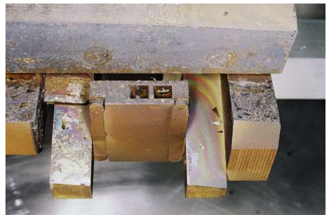
Fig. 50. Photograph of the inner carrier 2IN after removal in 2007. The bottom of Tile 3 is at the top of the picture. Surfaces are covered with a thick deposit, which is showing signs of spalling in certain places. The front face of the mirror test unit is so thickly coated that it is not possible to see where the third channel (with a sample flush to the face) is.
