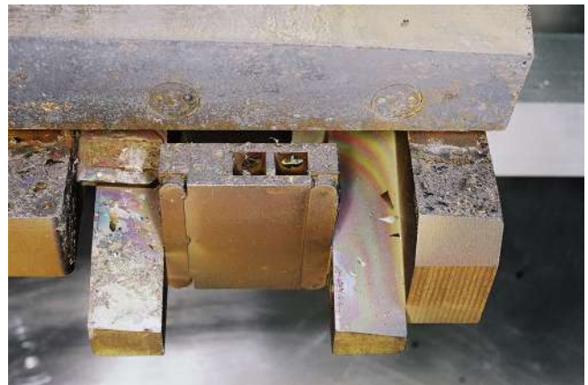
Fig. 50. Photograph of the inner carrier 2IN after removal in 2007. The bottom of Tile 3 is at the top of the picture. Surfaces are covered with a thick deposit, which is showing signs of spalling in certain places. The front face of the mirror test unit is so thickly coated that it is not possible to see where the third channel (with a sample flush to the face) is.
