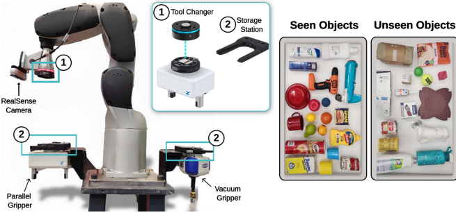
Fig. 5. Left: Our multi-gripper system with depth camera includes a parallel and vacuum gripper stored in dedicated stations (2). The automated tool changer (1) facilitates quick switching by connecting directly to the gripper and removing it from its station. Right: Real-world test objects.
