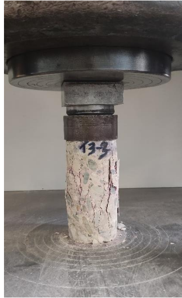
Figure 54: Typical failure mode of core specimens.
