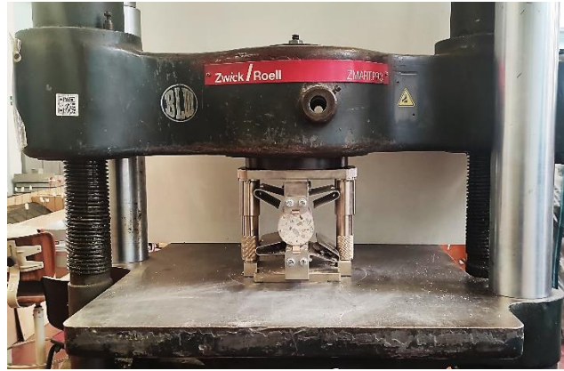
Figure 55: Tensile splitting strength test.
