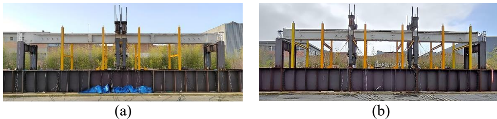
Figure 26: General view of test setup: (a) three-point loading configuration, (b) four-point loading configuration.
