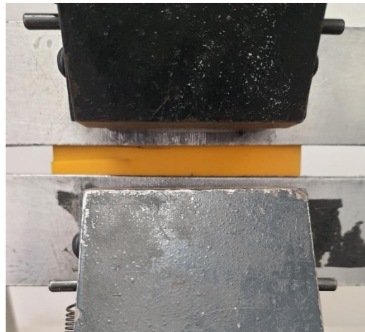
Fig 5. Pure shear specimen subjected to the uniform strain rate in testing machine
