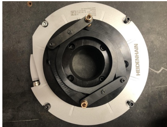
Figure 5. RCN encoder and the decoupling mechanical joint mounted on it.
