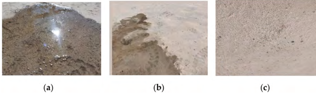
Fig. 9. Example of concrete curing category pictures: (a) The fully cured area; (b) The incompletely cured area; (c) The uncured area.
