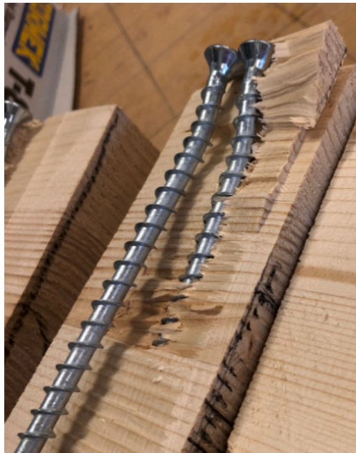
Fig. 2. Buckling failure of a screw loaded in compression.
