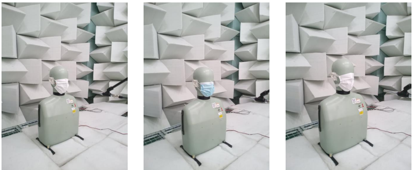
Figure 1. Face masks mounted on the head and torso simulator in the anechoic room of the Politecnico di Torino. From left to right: Mask 1, Mask 2, Mask 3.
