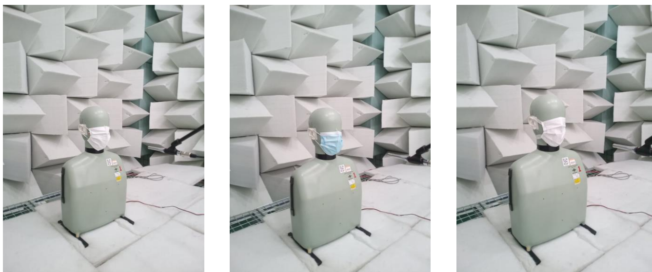
Figure 1. Face masks mounted on the head and torso simulator in the anechoic room of the Politecnico di Torino. From left to right: Mask 1, Mask 2, Mask 3.
