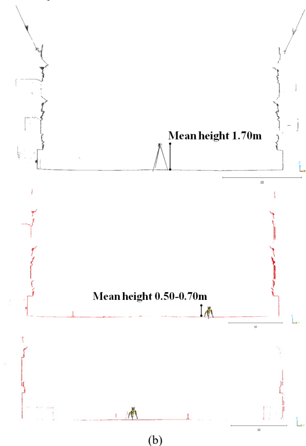
Figure 10. A transverse section of the courtyard point cloud, showing the capability of surveying the court pavement according to the sensor height for (a) TLS ground truth and the BLK ARC static dataset (b) side-trajectory and center trajectory.
