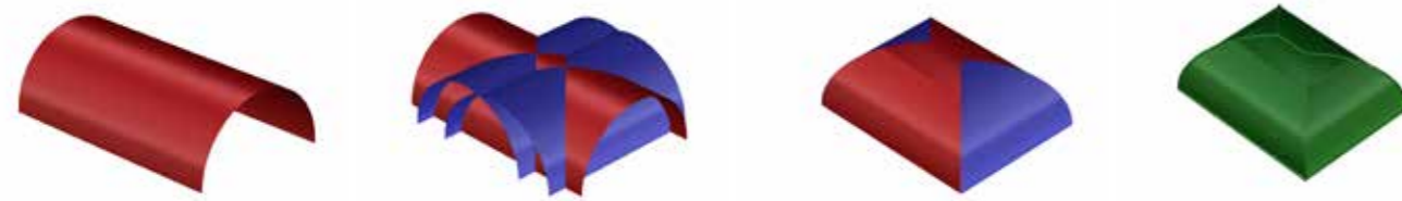
3b 1.4. (above): an internal view of the space of Hall C. (below) A classic geometric generation of a barrel vault with pavilion heads
