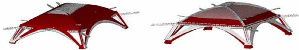
3b 1.12: Spatial comparison of the two 3D models, the red version derived from Nervi's original drawings, and the gray version derived from the terrestrial laser scanning survey. (left) Alignment based on floor level, (right) alignment based on impost vault level (elaborated by S. Perri I. Cofano)
