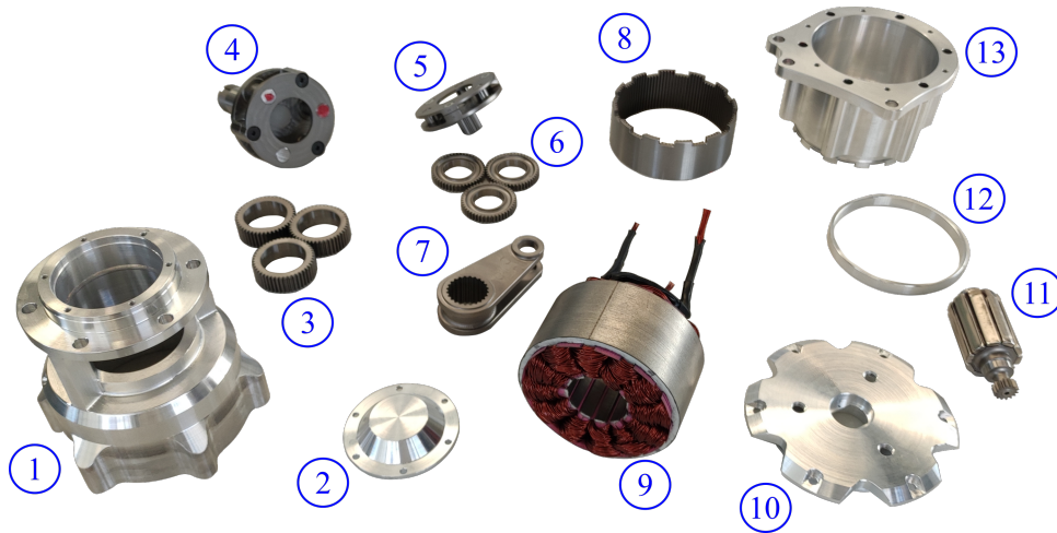
Figure 3.38: Components of the manufactured REmSA prototype for the motorcycle application. Gearbox: casing (1), cover (2), first stage planets (3) and carrier (4), second stage carrier (5) and planets (6), lever (7), ring gear (8). Electric machine: stator (9), cover (10), rotor (11), spacer (12), casing (13).
