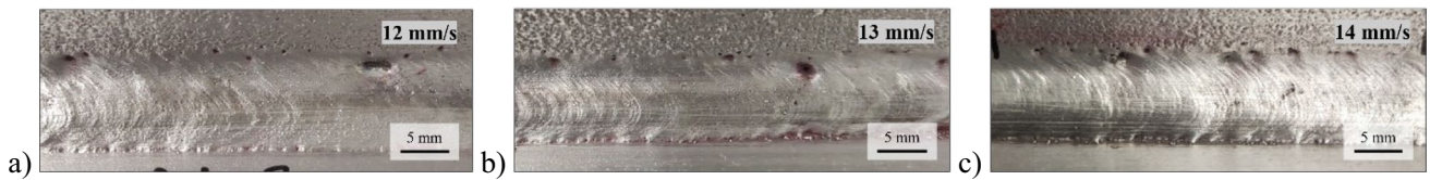
Fig. 3 Visual appearance of each sheet/cast GMAW joints carried out with a travel speed of a 12 \text{ mm/s} , b 13 \text{ mm/s} and c 14 \text{ mm/s}
