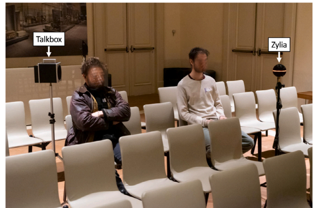
Fig. 3. Picture of the RIR recording procedure in case of Zylia placed in the farthest listening location w.r.t. the target speaker and the Talkbox placed in the respective 120° azimuth noise location.
