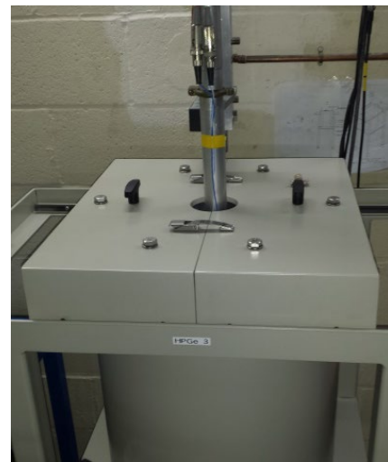
Fig. 3. KN2 transfer system at the counting station . Capsule inside the tube entering the lid of the low background lead shield to the detector within.
