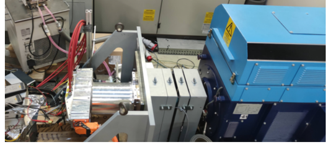
Fig. 13. Test bench for experimental TRL6 validation [6], including the full-scale integrated motor-inverter unit, torque meter and load machine.
