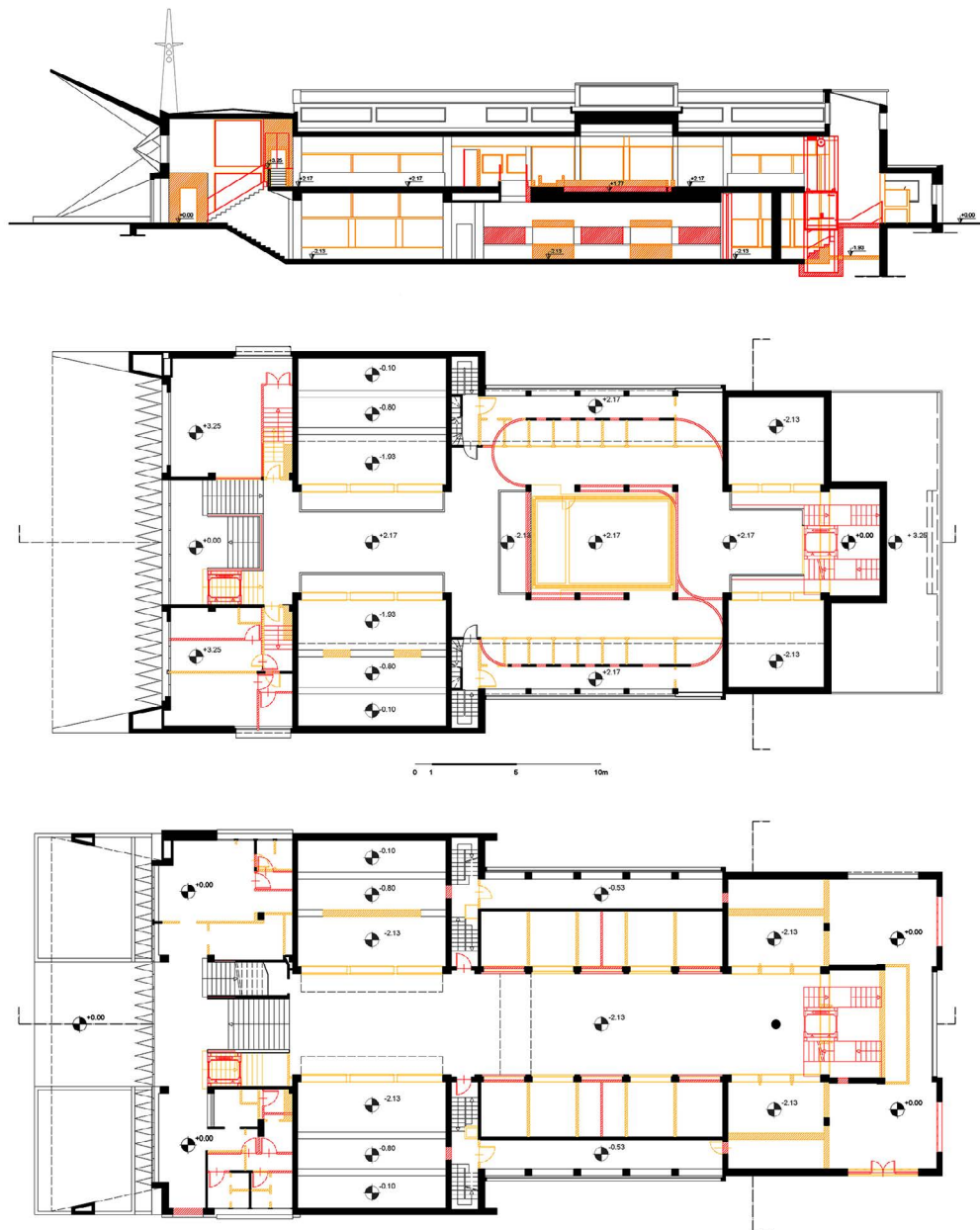
Fig. 5 - Demolition and construction for the Museum of Japanese Comics and Animation design project inside Enzo Venturelli's aquarium-retailarium. From the bottom ground floor, first floor, and longitudinal section view (Author: V. Bottari).
