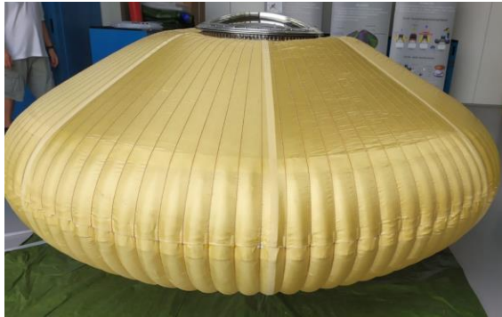
Figure 10: IS static inflation phase (prior to deflection).
