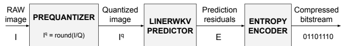
Fig. 1: Overview of compression scheme for near-lossless compression. A raw image is prequantized by means of a uniform scalar quantizer, then fed to a causal prediction model implemented by the LineRWKV neural network, producing prediction residuals that are entropy-coded.
