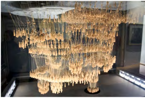
Fig. 1. Gaudi's Hanging Weights Model, picture courtesy eetthaannn available at: https://flic.kr/p/2g24Jcm (CC BY-NC 2.0).
