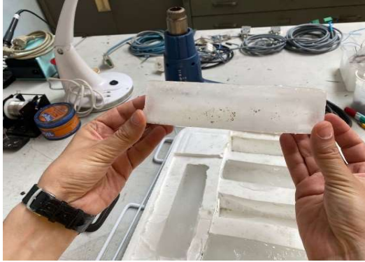
Figure 5– Resin mold and the plain ice specimen
