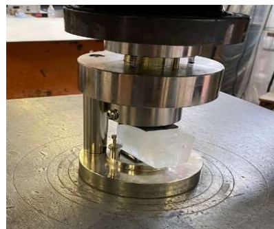
Figure 8– Compression test performed on ice (a): before the test (b): during the test.
