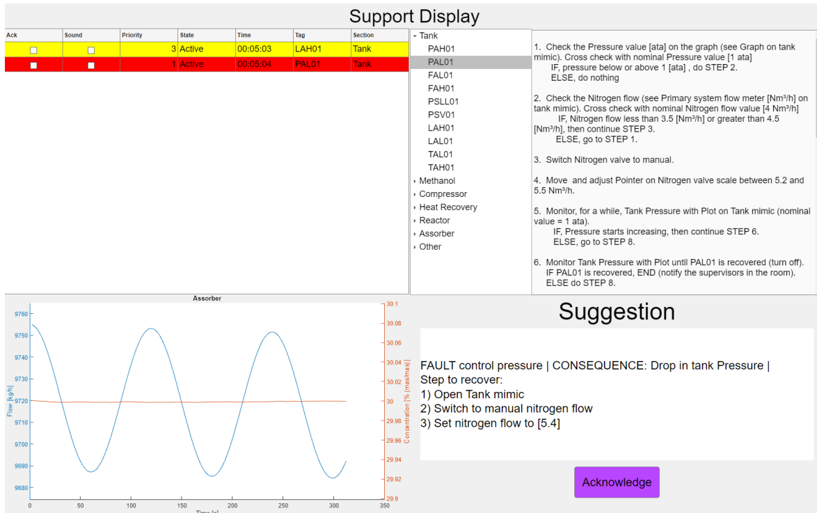
Figure 3. Support panel layout: In the upper-left quadrant, the alarm list alerts the operator to current issues. The upper-right quadrant houses the traditional procedure system. The lower-left quadrant features a critical graph displaying production metrics. In the lower-right quadrant, the suggestion box automatically provides situation-specific recommendations to the operator. First published in Lecture Notes in Computer Science vol. 14294, pp. 15–26 by Springer Nature, [30].
