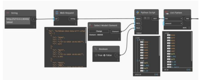
Figure 14. Dynamo script showing the connection of String , Web request , Python script and List flatten nodes.
