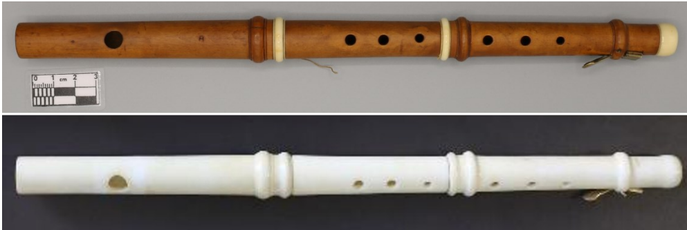
Figure 4.46: Original (top) and 3D printed (bottom) Piccolo Flute.
