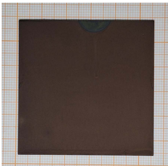
Fig. 7 Photograph of a large-area ( 5.3\text{ cm} \times 5.3\text{ cm} ) flat Crofer 22 APU interconnect coated and thermally treated.
