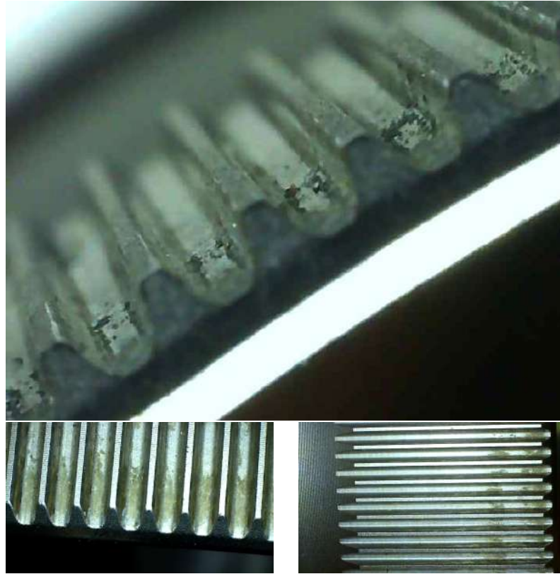
Figure 7. Wear of the flexspline teeth.
