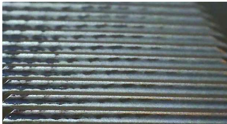
Figure 6. Effect of the coning angle on flexspline tooth wear.
