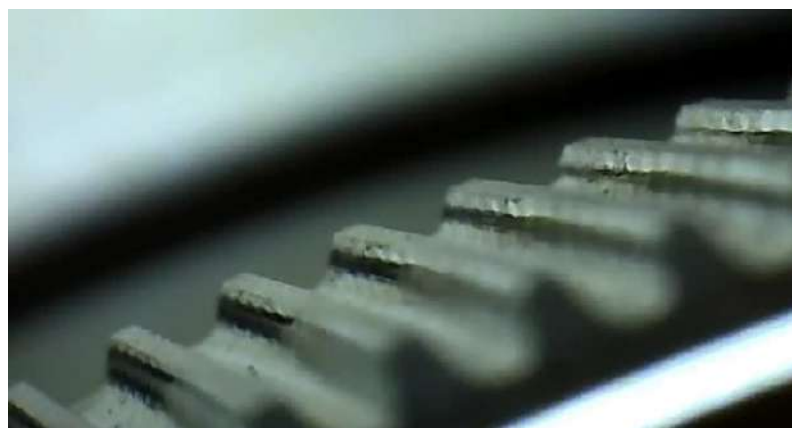
Figure 10. Flexspline tooth cracks.
