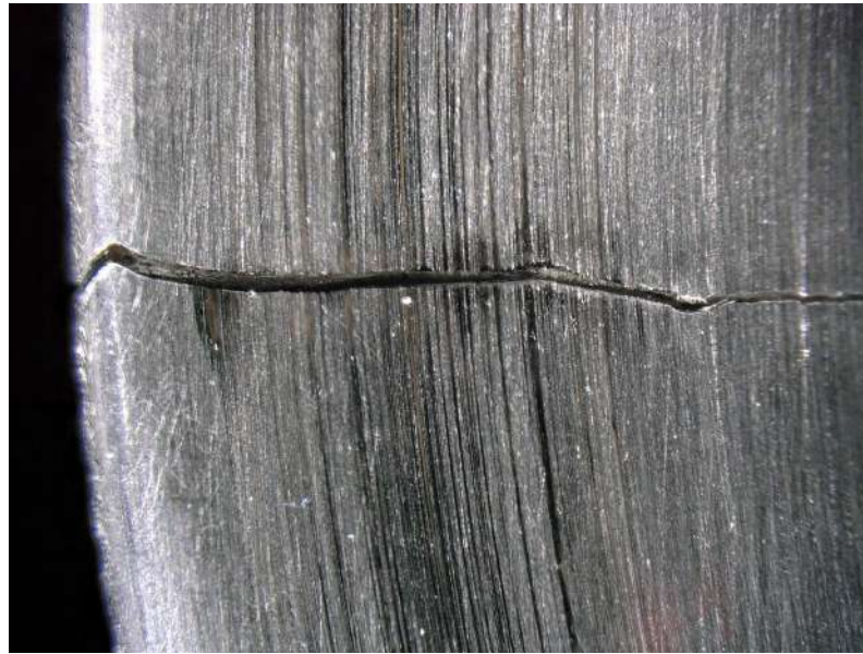
Figure 9. Crack in the FS rim.
