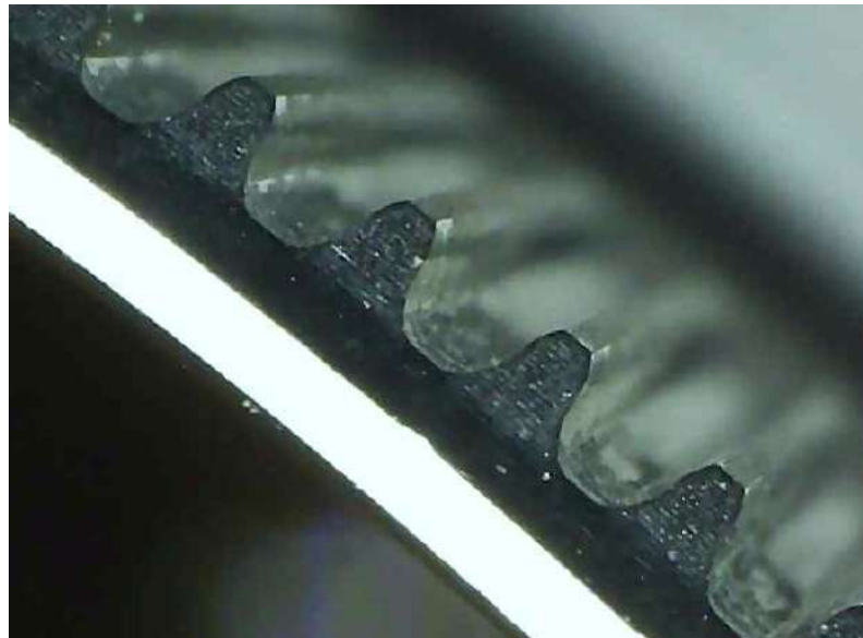
Figure 2. Double-arc profile of the flexspline tooth.
