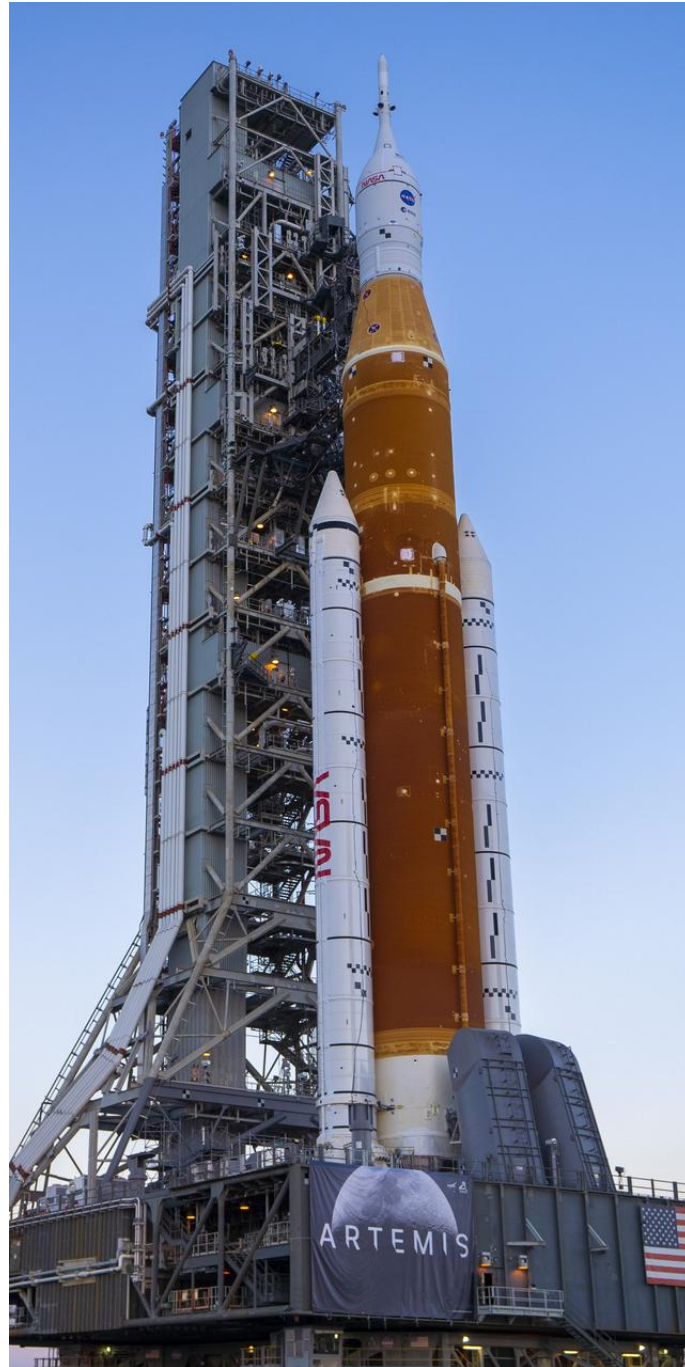
Fig. 1.1 Space Launch System close up at Kennedy Space Center. SLS Solid Rocket Booster derived from Space Shuttle Boosters are one of the prominent and latest application of SRM in the space launcher field (Credit to NASA/Sam Lott)
