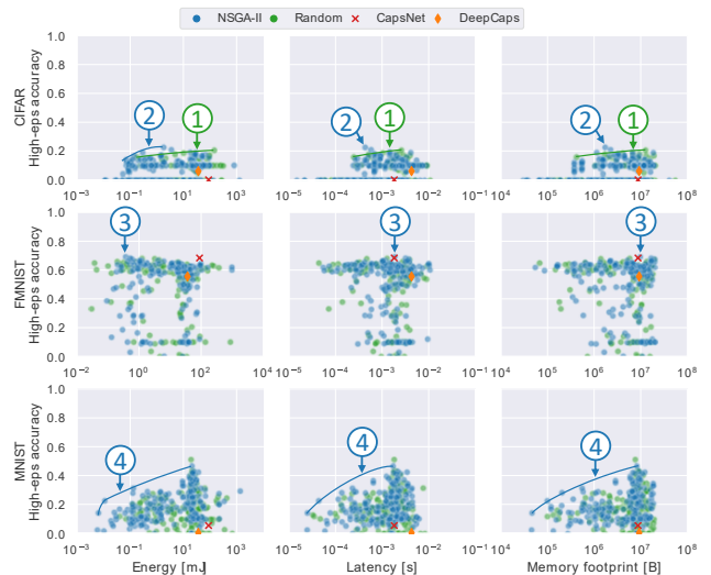
FIGURE 14: RoHNAS ' fast evaluation of DNN robustness under PGD attack in the Two EPS setting using the \epsilon_{high} value, compared to the solutions found with random search, showing tradeoffs w.r.t. energy, latency, and memory footprint.
