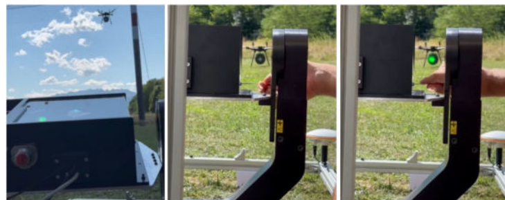
Figure 8. Optical alignment procedure illustrating mechanical adjustment of the beam with respect to the reference frame. (Left): Optical chain mounted on the pitch stage of the 2-axis gimbal while pointing toward the UAV using the green aiming laser. (Center) and (Right): Calibration of the Fine Steering Mirror through two micrometric adjustment screws, used to center the beam on the receiver panel after coarse pointing based on the RTK target position and the inverse kinematics solution.
