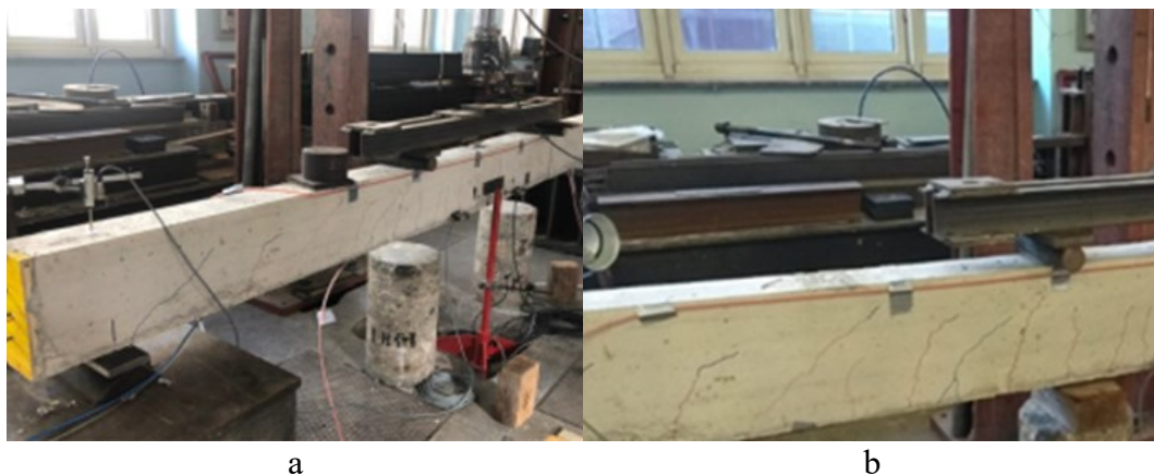
Figure 4. Test setup (a) and crack pattern at failure (b)
