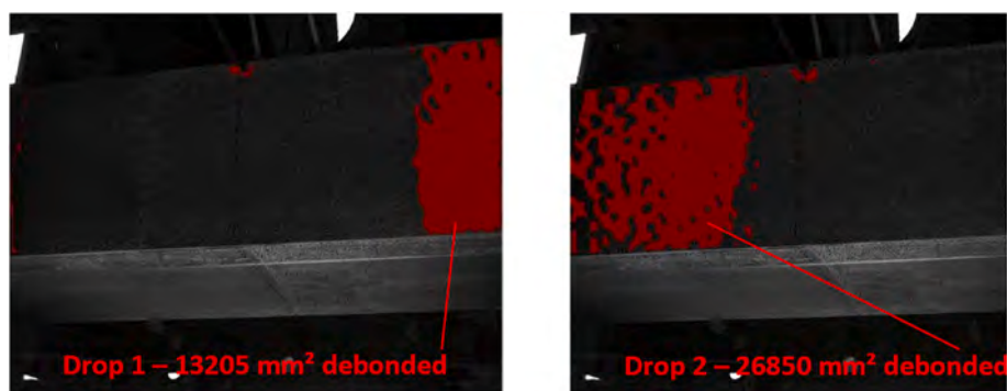
Fig. 22. Quantification of the debonding area of repairing TRC patch from concrete substrate by DIC strain difference before and after two load drops (Aggelis et al., 2016).
