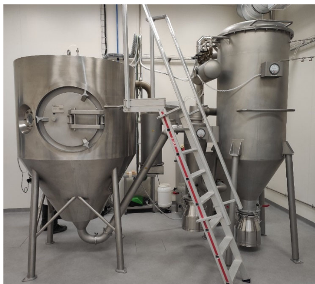
Figure 2.2: Industrial spray dryer used for the scaling-up trials.
