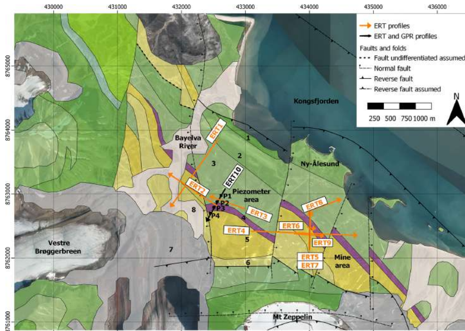
Figure 2. Geological map (data from NPI, WMS geological map at 1 : 250 000): (1) carbonate rocks of Wordiekammen Formation (Moscovian–Sakmarian); (2) carbonate rocks of Gipshuken Formation (Sakmarian–Artinskian); (3) chert, shale, sandstone, and limestone of Kapp Starostin Formation (late Artinskian – late Permian); (4) shale, siltstone, sandstone of Vardebukta Formation (Induan); (5) sandstone, shale, coal of Kongsfjorden Formation (Paleocene?); (6) sandstone, shale, conglomerate of Brøggerbreen Formation (Paleocene?); (7) moraine (Holocene); (8) glacio-fluvial deposits (Holocene); (NF) normal fault; (RF) reverse fault. The coordinate system is WGS84-UTM33N. The geological map was exported from the WebGIS tool by the © Norwegian Polar Institute ( https://geokart.npolar.no/Html5Viewer/index.html?viewer=Svalbardkartet , last access: January 2024).
