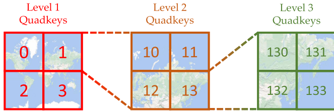
Fig. 3. Logic for the definition of Quadkeys on a Mercator projection of the world, as defined by Microsoft [25].
