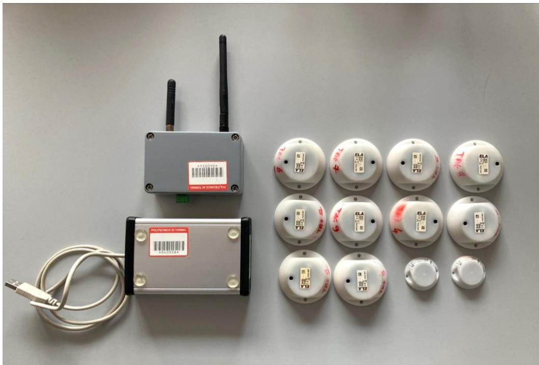
Figure 42: PUCK RhT sensors by ELA Innovation used for Experience II. From left to right: the antenna, a tag encoder, 10 RHT sensors, and 2 lux sensors
