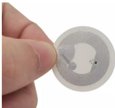
Figure 39: Adhesive NTAG tag used for experience
