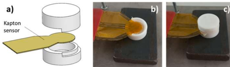
Fig. 8. (a) Special device for Hot Disk Test with grease; (b, c) Experimental setup.
