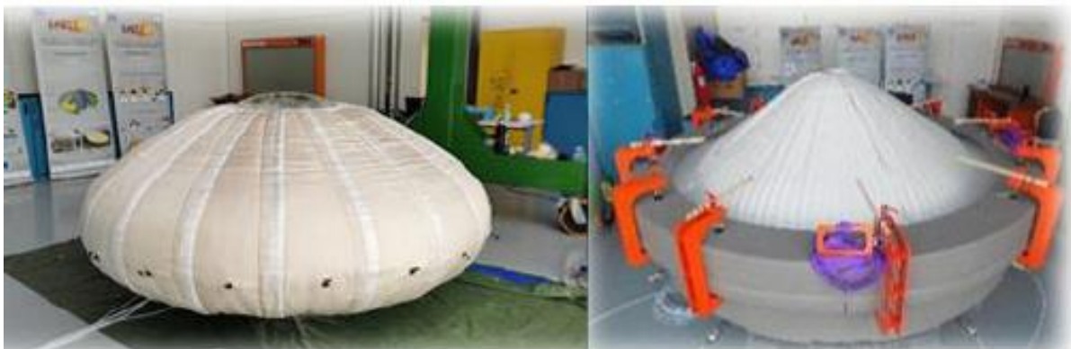
Figure 20 Static-load testing of the EFESTO inflatable heat shield ground demonstrator
