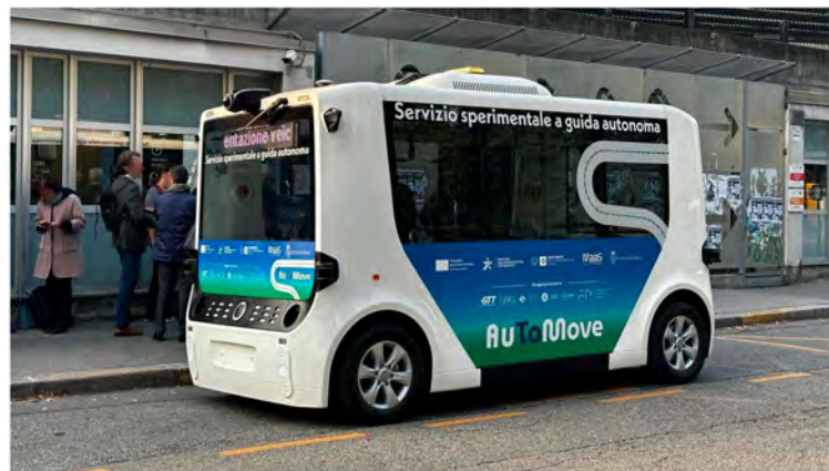
Figure 2. Ohmio LIFT low-speed automated driving (LSAD) shuttle used in the ToMove experimental service in Turin.
