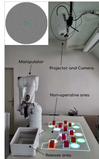
Fig. 2. NeuroTag (top-left) and the projected interface. The NeuroTags are positioned close to the objects to be picked up by the manipulator.
