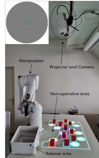
Fig. 2. NeuroTag (top-left) and the projected interface. The NeuroTags are positioned close to the objects to be picked up by the manipulator.
